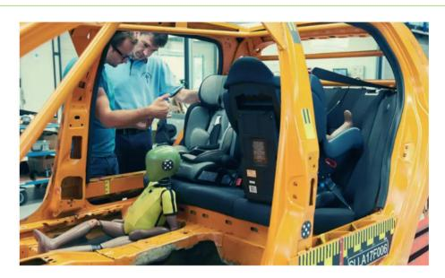
Fig. 5. Crash test frame of ADAC vehicle seats [8]
