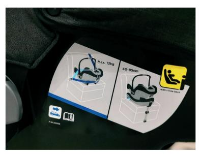
Fig. 2. Marking of the methods of mounting the child seat of the youngest group in a passenger vehicle
